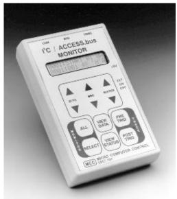
The MIIC-101 Bus Monitor is a Stand-Alone and Remote Troubleshooting Tool for the I2C (Inter Integrated Circuit) serial bus developed by Philips Semiconductor, or the System Management Bus (SMBus) developed by Intel, and other dervived protocols.
