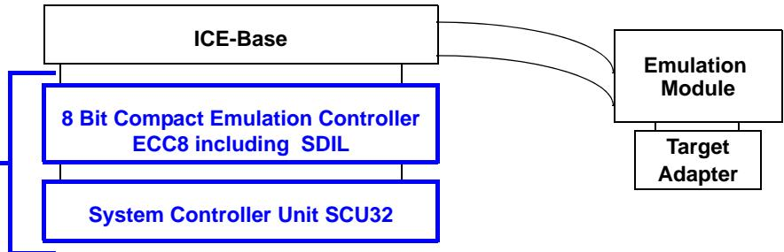
TRACE32<sub>COMPACT8</sub> is a cost effective compact solution for all supported 8-bit CPUs. It is entirely designed for the development of 8-bit target systems.
