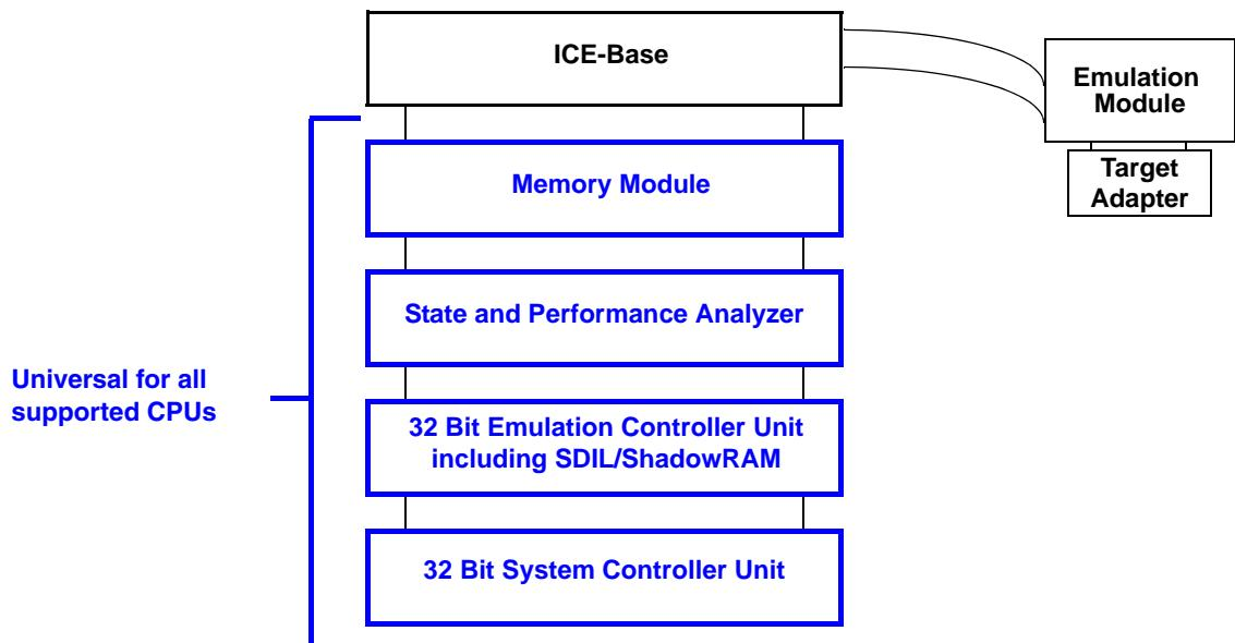
TRACE32-ICE uses a modular technology and consists of the following parts:
