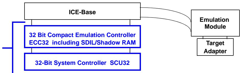
TRACE32<sub>COMPACT32</sub> is a cost effective compact solution for all supported CPUS. The 32 Bit Compact Emulation Controller is a high integration of the 32 Emulation Controller ECU32 and the State
