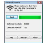
Simply insert the analyzer into the active connection, press 'scan' and after having decoded some characters you will get information about the probable data format.
